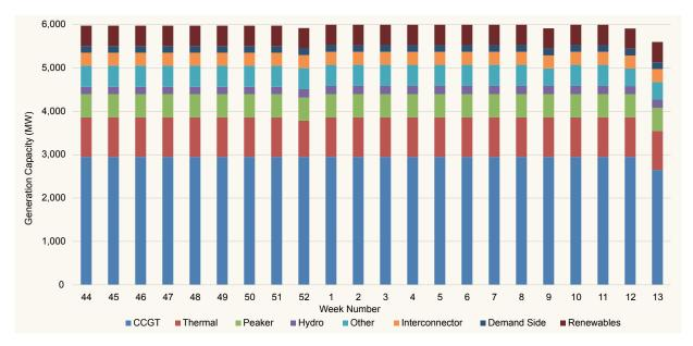
Figure 13: Ireland expected weekly de-rated generation capacity per type of generating unit
