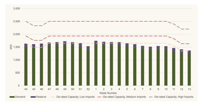
Figure 7: Northern Ireland weekly de-rated generation capacity based on the largest unit being unavailable (dashed lines) for each import scenario versus the forecast demand plus reserve (bars)
