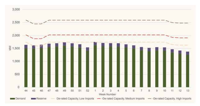
Figure 6: Northern Ireland weekly de-rated generation capacity based on de-rating factors (dashed lines) for each import scenario versus the forecast demand plus reserve (bars)
