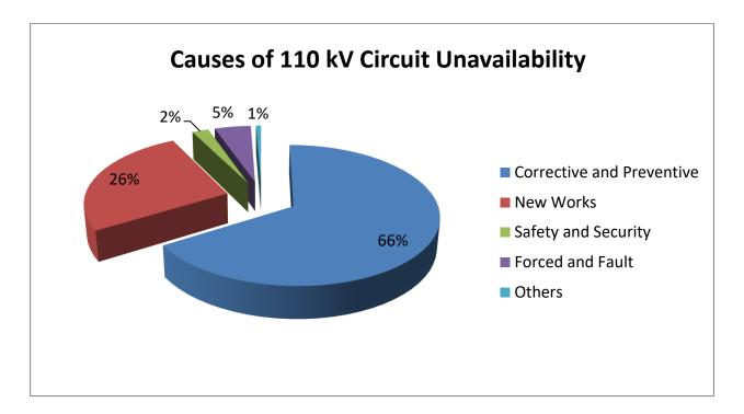
Figure 10: Causes of Unavailability on the 110 kV System in 2022
