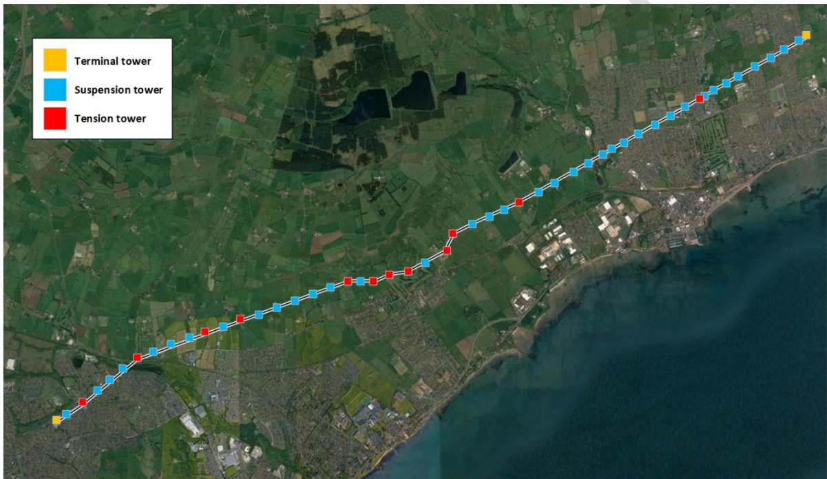
Figure 2.3: Carnmoney to Eden 110 kV double circuit route
